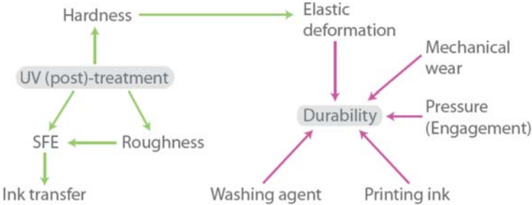
Figure 8. Influencing parameters in flexography related to printing plate
