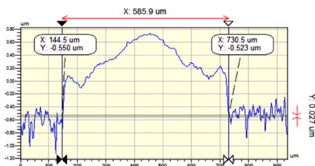
Fig.19. Cross section and width of the printed fine line measured by white light interferometry
