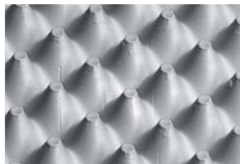
Fig.1. MacDermid LUX ITP 5% dots at 150 lpi
