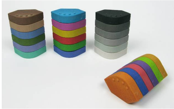
Figure 126. Example of custom designed colour test object, 3D printed colour test blocks (Walters, XX)
