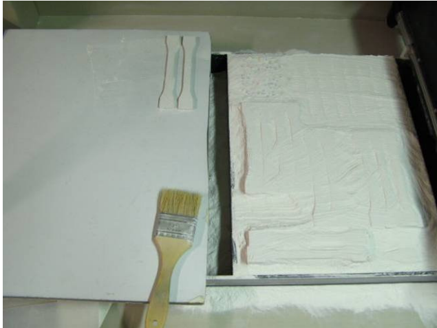
Figure 14. Post-processing, gross de-powdering, ZPrinter 510
