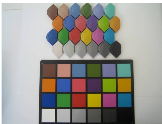
Figure 125. Example of printed custom designed 3D colour test object, with the respective GretagMachbeth ColorChecker patches shown (Walters, XX)
