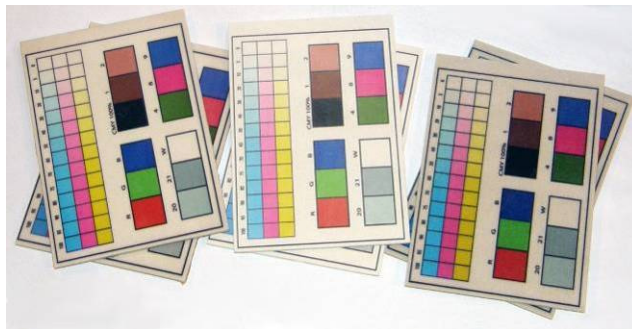
Figure 119. Custom colour charts, infiltrated with cyanoacrylate (left), non-infiltrated (middle), infiltrated with epoxy resin (right)
