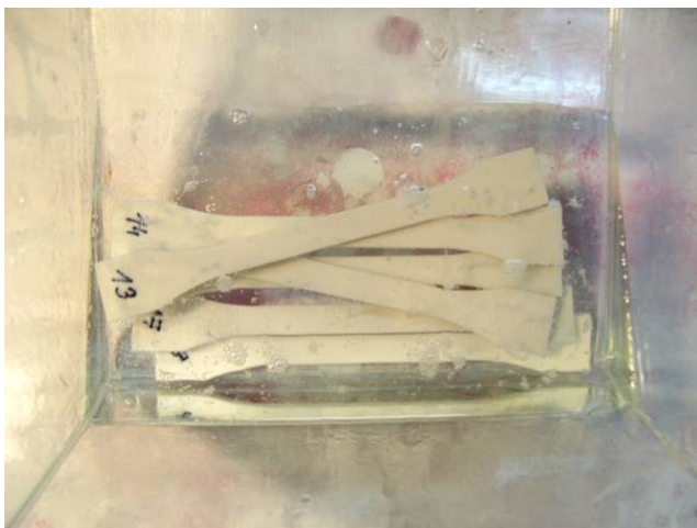
Figure 16. Post-processing, example of finishing by dipping in infiltrant
