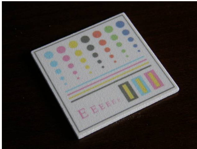
Figure 27. Example of printed and post-processed test plate
