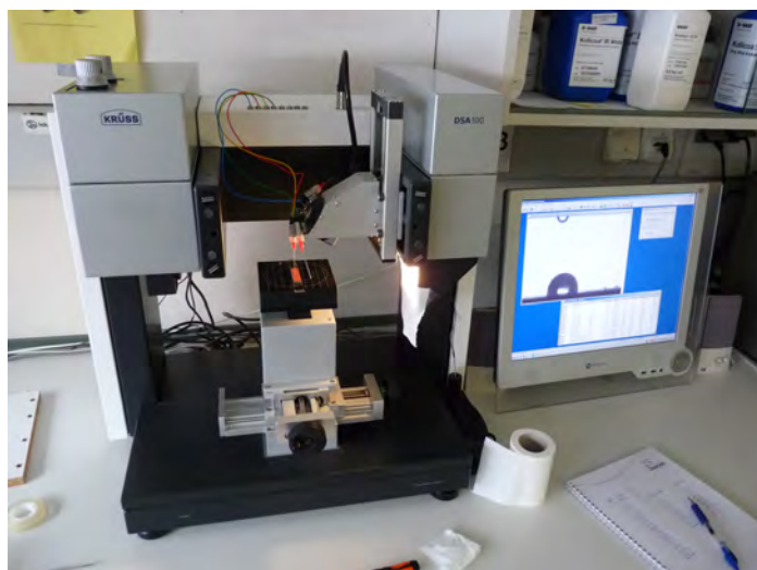
Figure 14: Krüss DSA 100 apparatus during measurement of RED sample.
