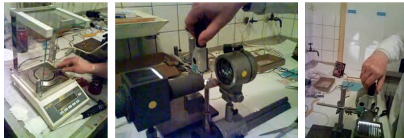
Figure 23: Process (from left to right) of weighing, splitting flexographic printing ink droplet and projection of split droplet onto the screen to control the experiment.
