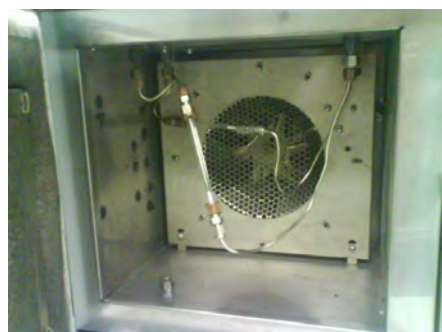
Figure 21: Measuring chamber of Agilent Technologies 6890N, glass cylinder filled with silica, connected to gas inlet and measurement sensor is visible.
