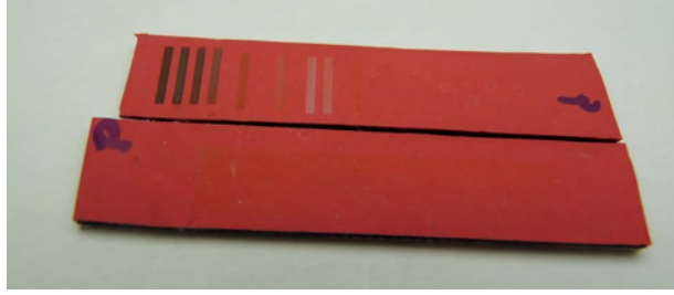
Figure 13: Steps to achieve JND on RED plasma treated sample by rendering 8 \times 1 mm area with different settings of UV laser device (top) and rendered surface 8 \times 40 mm for final sample (down).
