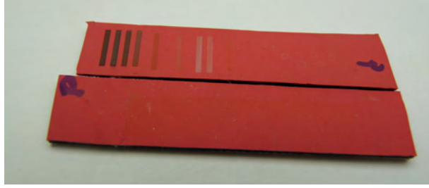
Figure 13: Steps to achieve JND on RED plasma treated sample by rendering 8 \times 1 mm area with different settings of UV laser device (top) and rendered surface 8 \times 40 mm for final sample (down).
