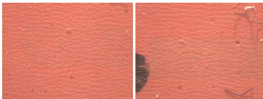
Figure 57: Rough waviness structure on RED sample, untreated (left), oxygen plasma and JND IR laser treated (right), visible only under narrow lighting angle from side, perpendicular to the waves. Same structure is not visible on SEM images.
