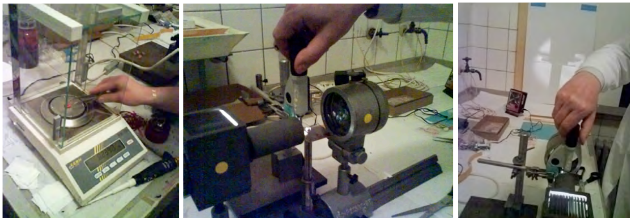
Figure 1: Process of weighing, splitting of flexo printing ink droplet and projection of splitted droplet at the screen to control the experiment (method of M. Kaplanová).
