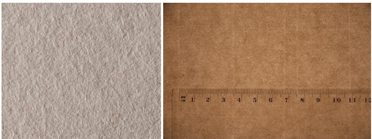
Figure 1 - Model paper's surface under raking light (left) and its chain lines captured in transmitted light (right).
