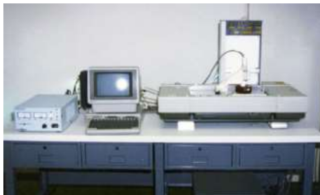
Slika 28: Prvi 3D printer SLA 1 preuzeto s: https://www.sculpteo.com/en/3d-learning-hub/basics-of-3d-printing/the-history-of-3d-printing/
