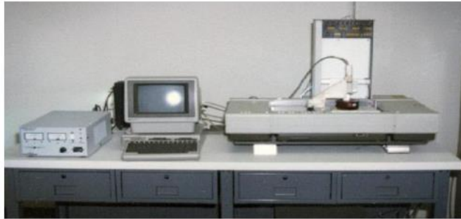
Slika 1 - SLA-1 prvi komercijalni 3D printer (izvor: https://3dprint.com/72171/first-3d-printer-chuck-hull/ )
