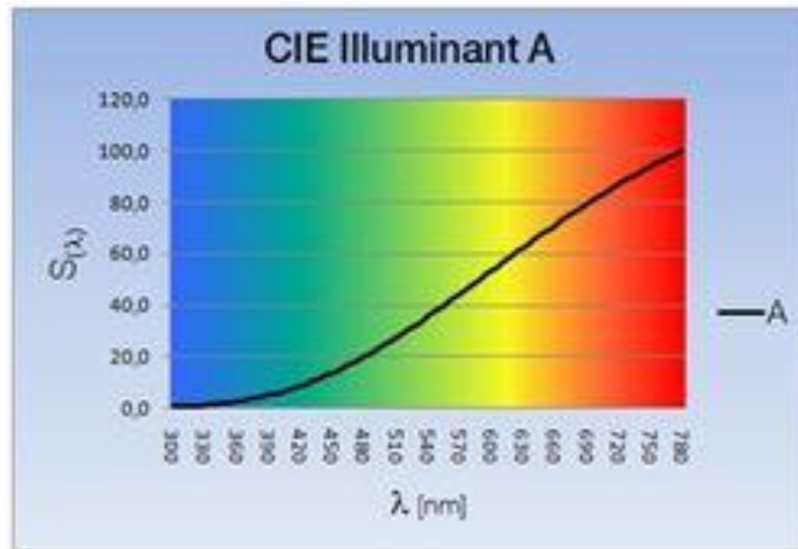
Slika 14 CIE Iluminant A (preuzeto sa : http://www.konicaminolta.eu/en/measuring-instruments/learning-centre/light-measurement/light/light-sources-and-illuminants.html )
