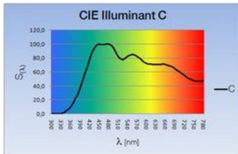
Slika 15 CIE Iluminant C (preuzeto sa : http://www.konicaminolta.eu/en/measuring-instruments/learning-centre/light-measurement/light/light-sources-and-illuminants.html )
