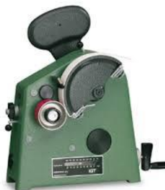
Slika 2. IGT A1 and A2 printability testers. [9]
